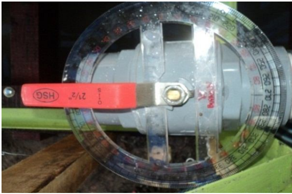
Fig.4 Ball valve with 90° shut-open
